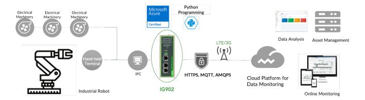
The industrial robot on the production site consists of the robot, the hand-held terminal and the control system. Via high-speed Ethernet, the core control system is connected to the IG902 which collects data of the robot's operation status, such as the axis set velocity, axis feedback velocity, axis accelerated velocity, axis feedback location, axis alarm code, temperature of the electrical machinery, shaft torque, etc.
